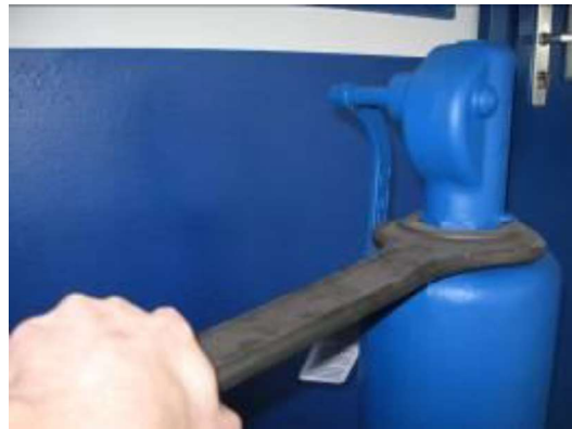
Fig. 3 Installation of the lever and cap
