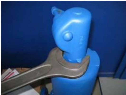
Fig. 3 Installation of the lever and cap
