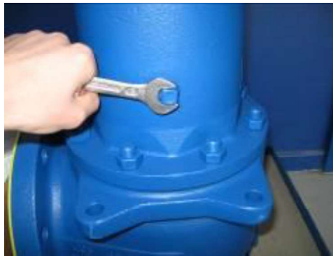
Fig. 2 Sealing the drain hole
