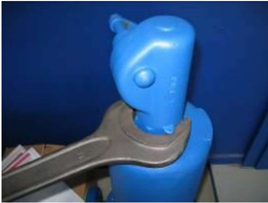
Fig. 3 Installation of the lever and cap
