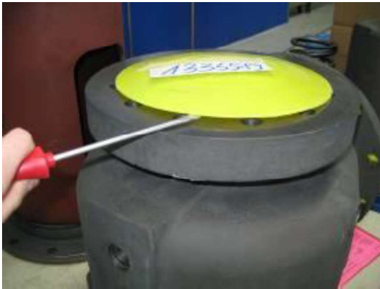
Fig. 3 Lifting the protective cap
